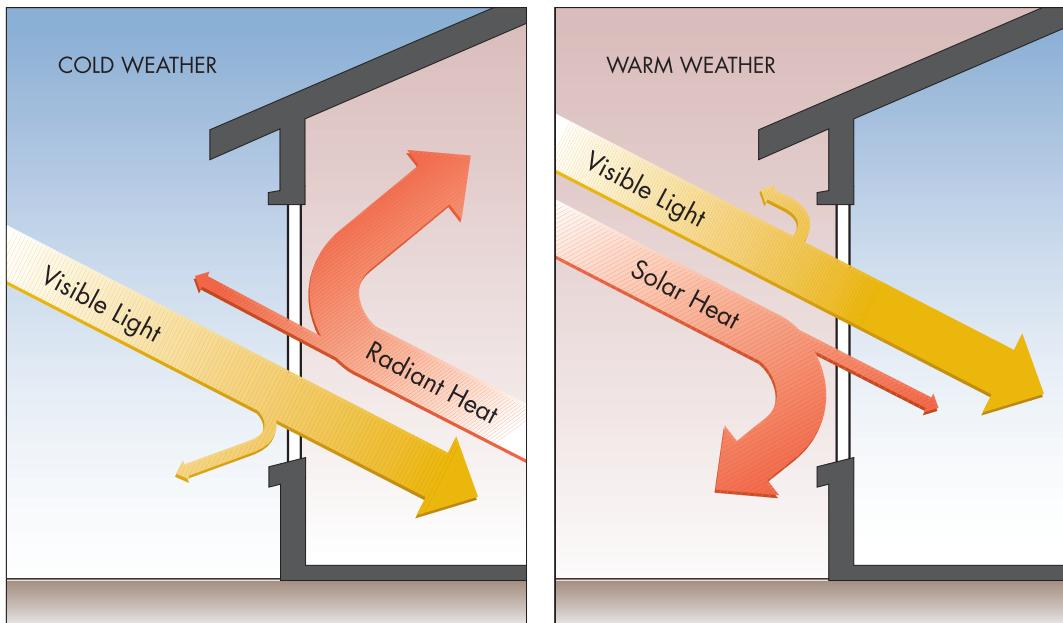
In cooler conditions, the Thermaflex coating reflects heat back into your rooms, while allowing a high level of visible light to pass through and be absorbed to add desirable extra heat to the room.
